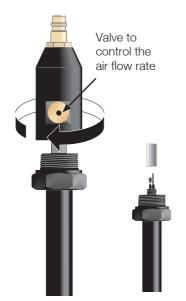
Place the measuring chamber on the humidity probe adapter and screw on tightly by hand.
