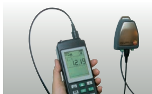
Inspection of transmitters with 4 to 20 mA interface
