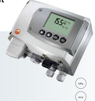
The differential pressure transmitter testo 6351 was developed specially for monitoring differential pressure in the measuring range from 50 Pa to 2000 hPa. For this reason, it is suitable for monitoring cleanrooms as well as for demanding VAC monitoring. In addition to this, the flow velocity or the volume flow can be calculated from the measurement of the differential pressure in a Pitot tube.
